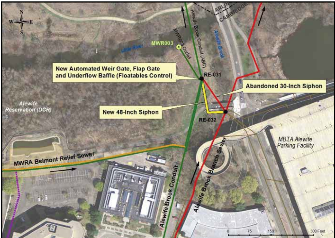
Figure 3: Control Gate and Floatables Control at Outfall MWR003 and MWRA Rindge Ave. Siphon Relief
