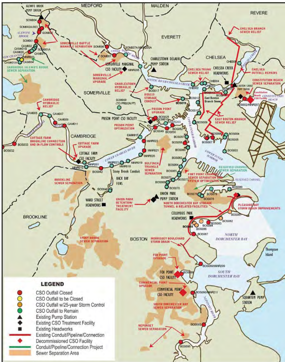
FIGURE 11-1 Approved CSO Control Plan and Status of Project Implementation (Complete projects in red; remaining projects in green)
