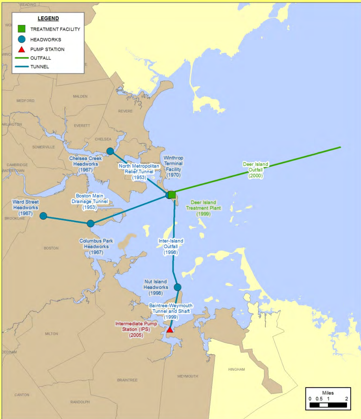
FIGURE 8-1 Headworks & Harbor Tunnel Location Plan
