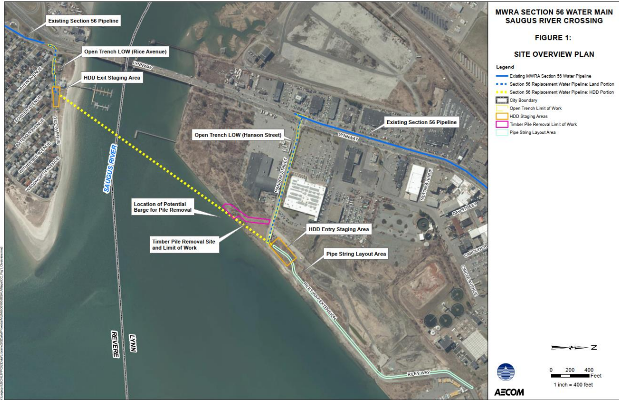
Figure 1. The proposed pipeline route, including two terrestrial portions (Lynn and Revere), and the section beneath the Saugus River. The terrestrial portions of the proposed water main will join with the existing Section 56 pipeline at the ends of Hanson Street and Rice Avenue.
