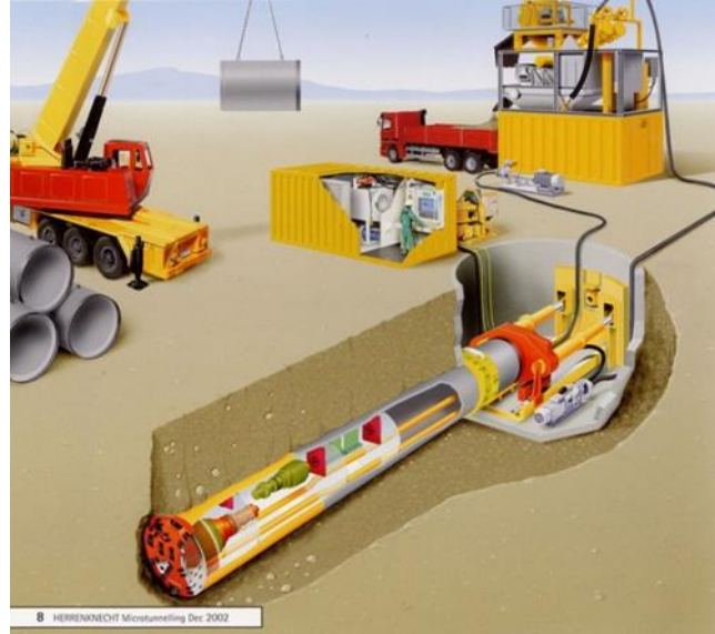
Figure 48 - Typical Microtunnel Operation
