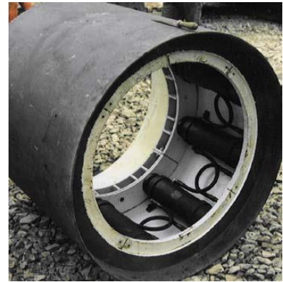
Figure 49 - Intermediate Jacking Station
