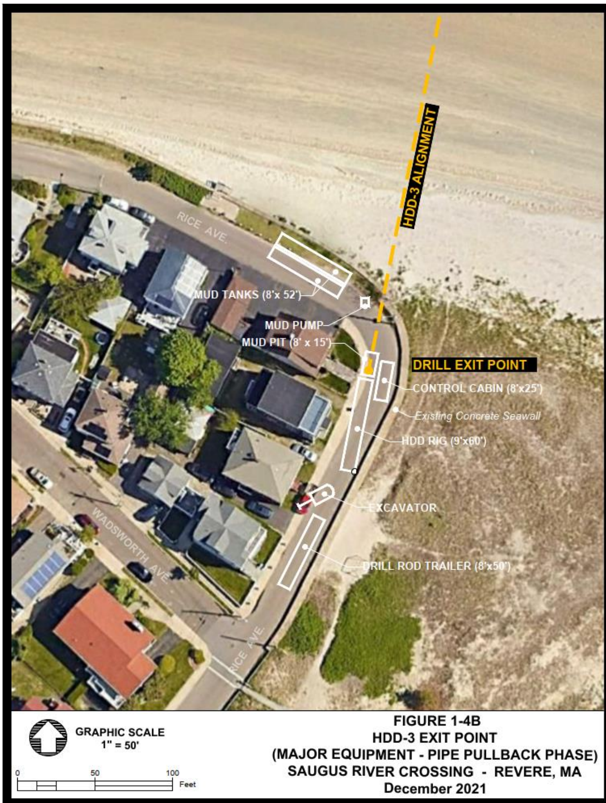
Figure 3 - Equipment Staging for HDD Route 3
