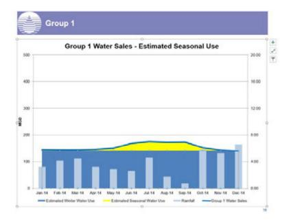
Carl continued to explain that Group 1 accounts for 73% of MWRA sewer flows. The green delta pictured in the graph below is the estimated inflow and infiltration (I/I): water from sump-pumps and down spouts and leaks into the pipes, respectively. I/I is typically greater when it rains, but after dry periods, the ground will absorb more water. Additionally, I/I may increase when rain occurs with snow cover.
