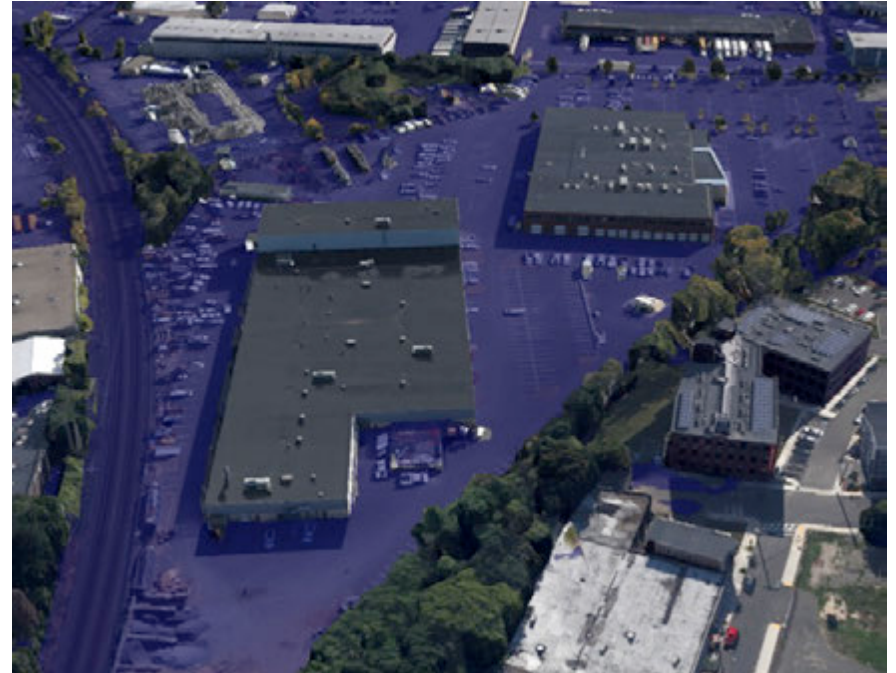
FEMA 100 Year Flood Elevation + 2.5ft
