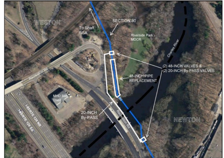
Figure 2- Section 80 Repair Site Map
