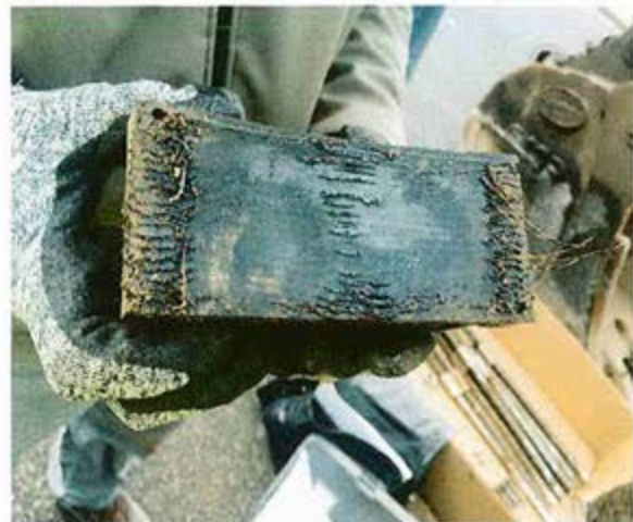
Failed flex restraint
