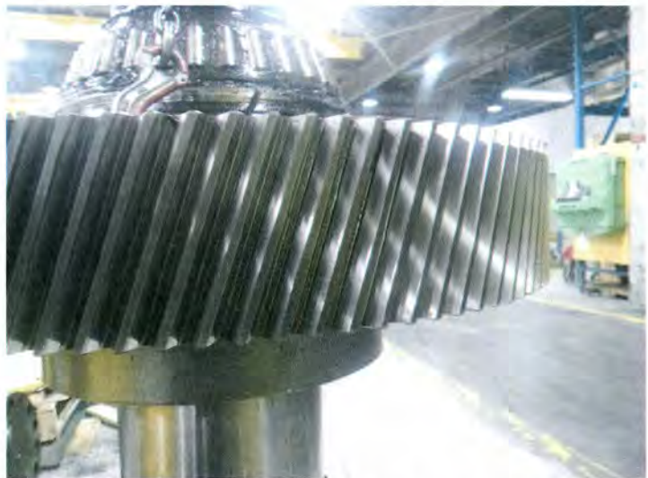
From Vendor's report, low-speed gear found with good wear pattern, suitable for reuse
