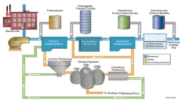
Water is flushed through a building's pipes into customer community sewers. These 5,100 miles of local sewers transport the wastewater into 227 miles of MWRA interceptor sewers. The interceptor sewers, ranging from 8 inches to 11 feet in diameter, carry the region's wastewater to two MWRA treatment plants. Most communities' wastewater flows to the Deer Island Treatment Plant with the Clinton Wastewater Treatment Plant serving the town of Clinton and the Lancaster Sewer District.
