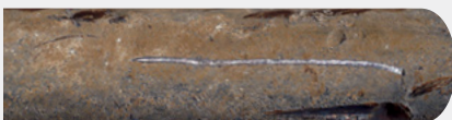
You can identify lead service line by carefully scratching with a key.
