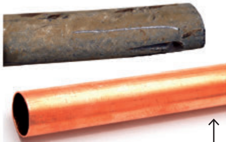
New Copper Service Line
