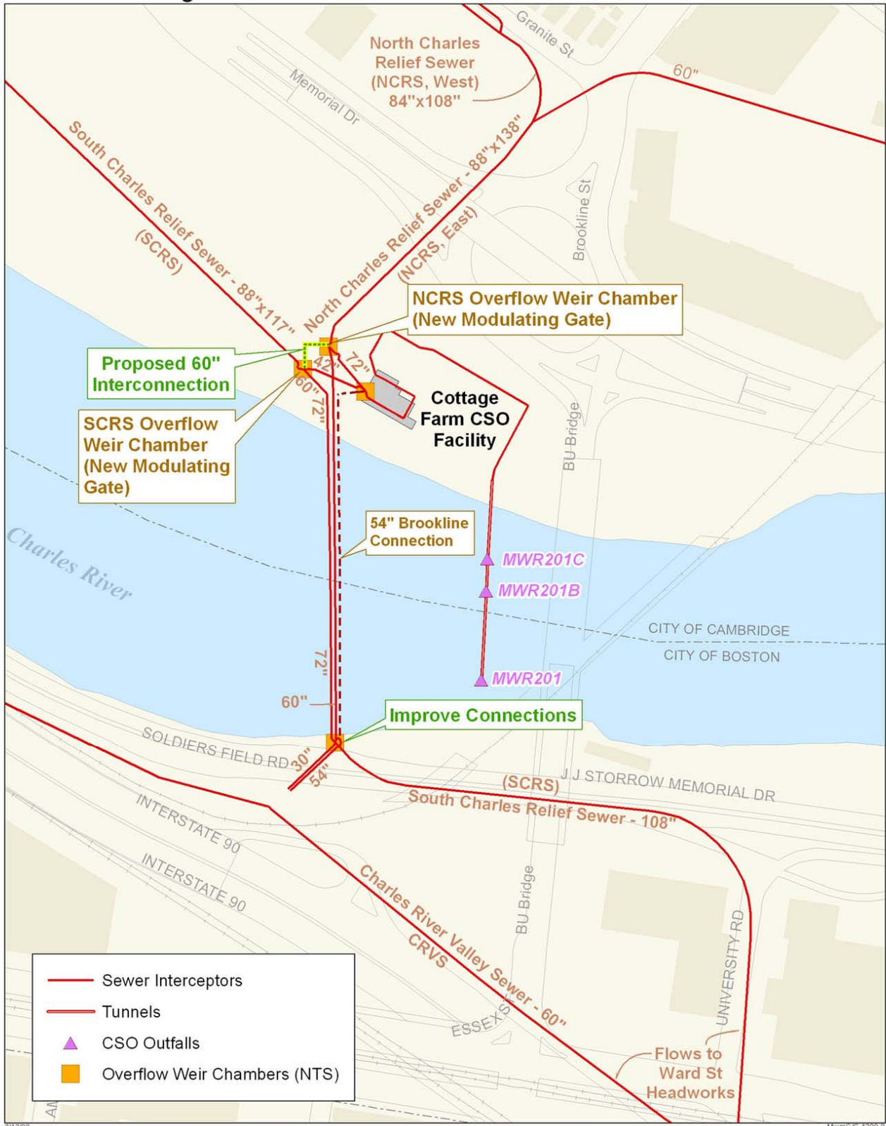
Figure 13 Cottage Farm Brookline Connection and Inflow Controls
