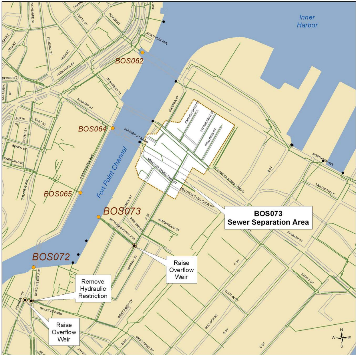
Figure 18 Sewer Separation and System Optimization for BOS072-073
