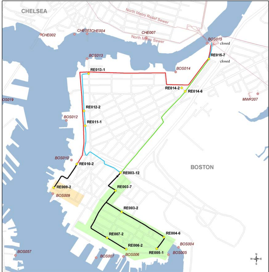
Figure 8 East Boston Branch Sewer Relief Hydraulic Relief with Sewer Separation Jeffries Point and Maverick Square (South)
