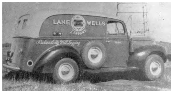
FIG. 1.—RADIOACTIVITY WELL-LOGGING INSTRUMENT TRUCK. Radioactivity monitoring instruments would be lowered down a well casing to categorize soil layers
